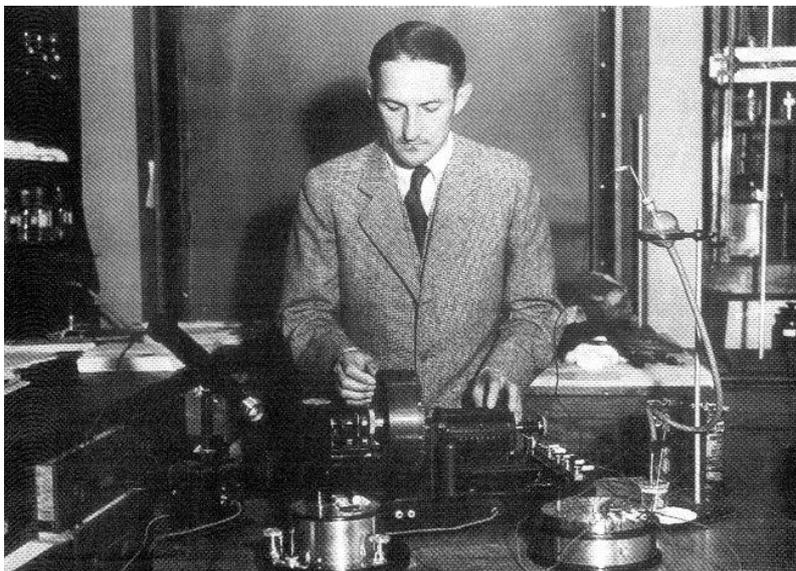
surface tension of polarized mercury by weighing drops of mercury from dropping mercury electrode. Next day after the examination Heyrovský visited Kučera's laboratory to get acquainted with his experimental set-up and the satisfied professor advised the student to continue in research of the method. Heyrovský replaced collecting, counting, drying and weighing the drops of mercury by measuring the drop-time, which is also proportional to surface tension. He found that from electrocapillary
