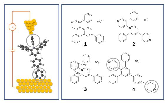
**Metal-molecule-metal junction for molecular electronics.** Metal-molecule-metal junction in the electric circuit arrangement (left) and molecular systems studied (right). Anchoring groups are indicated by gray circles.
