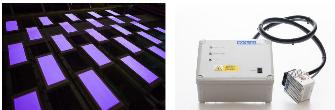
Figure 1. a) A roll-to-roll setup featuring 25 RPS400 planar plasma units, each with a plasma area 8 cm × 19 cm, operating in ambient air conditions, b) portable plasma unit RPS40+ (5 cm × 2 cm), utilized in [3].
